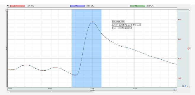
You have to define the limits for an acceptable transformation. In this example, the peak-to-peak measurement after smoothing and low-pass filtering at 1Hz differs by about 3% from the raw data (0.337 vs 0.347). But a filter this aggressive will eliminate most fast motion artifacts. If this trade-off is acceptable it's the researcher's decision and we recommend to always perform testing on both clean and noisy data before choosing a strategy to remove artifacts.
