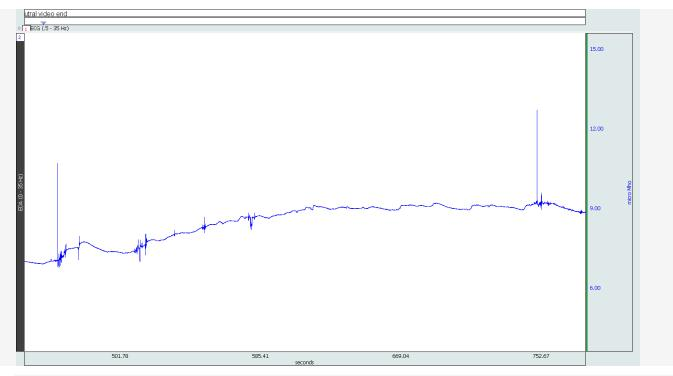
Next, we have resampled the data to 50Hz and applied a 50-sample median smoothing filter (Transform->Smoothing) and then 1 Hz FIR low pass filter (Transform->Digital filters->FIR filter->Low pass). We have zoomed in and the original data is seen on top with the transformed result on the bottom. The artifacts are completely eliminated:
